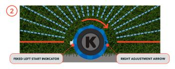
Rotate the ring with the right adjustment arrow to the right-most edge of this space. The rotary nozzle will apply streams of water between the left indicator and right adjustment arrow.
